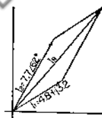
Fig. 7.3. Composition of Electric Current Vectors
